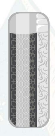
Preliminary filtration to remove sand, mud, rust & suspended solids.
